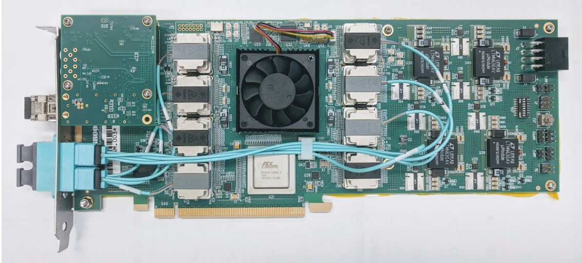
Figure 5.2: Photo of the CRI1 board (BNL-712 v2). The Kintex UltraScale FPGA is hidden below the black fan. It is surrounded by 8 Avago MiniPod transceivers, which interface to the optical fibers. The optical coupler on the left hand side consists of two MTP-48 connectors. The mezzanine PCB in the top left holds the interface to the TFC system. A PCIe switch combines the two SLR of the FPGA to the PCIe Gen3 x16 interface. The board is powered by voltage converters located on the right hand side of the PCB.
